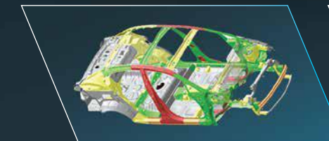
Reinforced Body Structure with Hot Press Formed Steel
